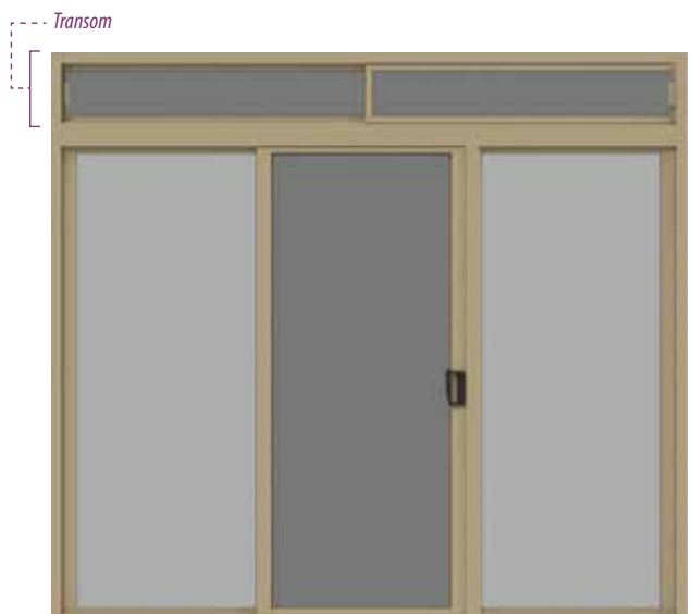
D3T Triple panel center sliding patio door with glass, screen & transom Widths from 96" to 124" | Door heights from 78" to 88" Overall door heights including Transom up to 120" Transom height with fixed glass or aluminum 10" to 36" Transom height with sliding glass 14" to 36"
