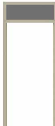
D1T/screen Frame for storm door with screen-only transom
